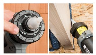
**12. Fill joints (line application)** Turn the ring under the spray nozzle to the "Line application" position and fill the joint with a line of sealant.
