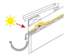
6c. UV protection for the membrane at the eave
