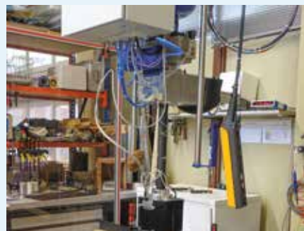
Fig. 32: Hail resistance test. Membranes can be bombarded with hailstones at speeds of up to 110 km/h from a hail launcher.
