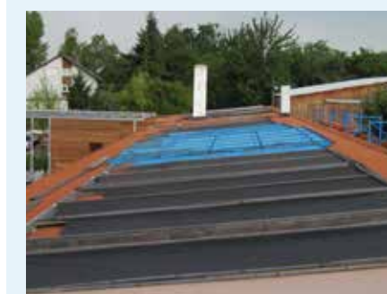
Fig. 34: Test set-up for outdoor exposure to investigate ageing resistance under direct exposure to the elements.
