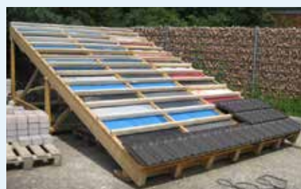
Fig. 37 a/b: Test roof to investigate the ageing resistance of underlay membranes under service conditions with a roof covering.
