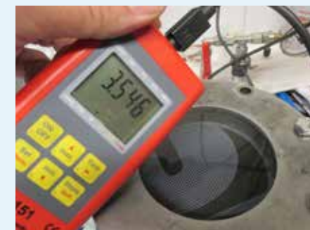
Fig. 23 a/b: Hydrostatic pressure test in the laboratory – overpressure is created using compressed air to simulate an artificial water column. Good-quality underlay membranes achieve values of over 2,500 mm.
