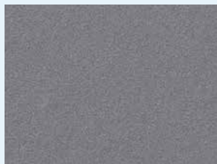
Fig. 15: Monolithic membrane – Microscope image with 1,000x magnification, closed/pore-free functional layer.
