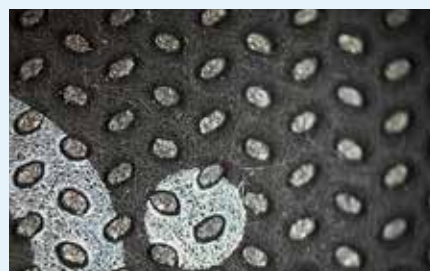
Fig. 36: Microscope images of a SOLITEX MENTO 3000 underlay membrane after 24 weeks of outdoor exposure – no damage can be observed.
