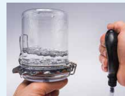
Fig. 17: Test bottle as a simple method of detecting the presence of micropores – pressure is applied underneath the membrane using a hand-held pump; if micropores are present, air will pass through the membrane and rise up in the form of bubbles.
