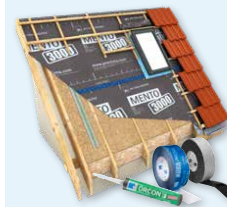
Fig. 45: Underlay membranes and accessories – associated products may be necessary to seal joints, tape over overlaps and seal nail penetrations; ideally, system components provided by the membrane manufacturer should be used.
