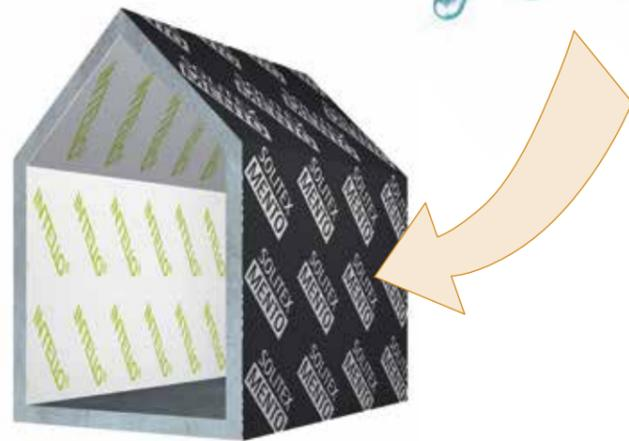
+ SOLITEX MENTO PLUS / ULTRA: extremely robust thanks to reinforcement: suitable for blown-in insulation materials
