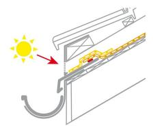
6c. UV protection for the membrane at the eave
