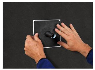
**1. Pull pipe/cable through** Clean the subsurface, then pull the grommet over the pipe or cable.
