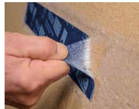
The primer strengthens unstable subsurfaces.
