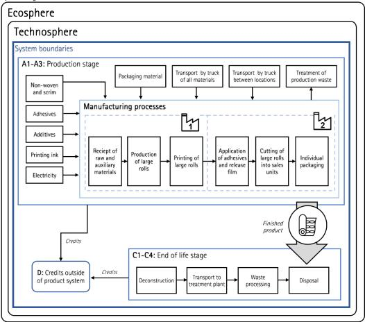
Each processing step within the system boundaries is marked with an icon and number (#1, #2, etc.), indicating the specific production site where it occurs. The system boundaries cover the following modules:
